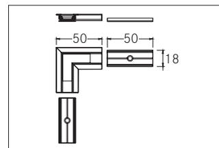
Connection piece 90°, white. Material: Aluminium, dimensions profile: length: 50 mm x width: 50 mm x height: mm .
