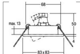
recessed spot, chrome, square. In a compact design, for installation in tool-less rapid assembly systems. . Lamp holder: GX5.3, Mounting method: Flush mounting, Place of installation: Ceiling-mounted, material: Steel, IP protection class: according to DIN EN 60529 IP20, Protection class: (EN 61140) III, voltage: 12V, Power: max. 50 W, Adjustability: swivelling, Energy efficiency class: A+ to C,
