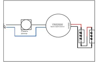
LED-Rundkonverter 350 mA, Phasenabschnitt dimmbar. . material: Plastic, IP protection class: according to DIN EN 60529 IP20, Protection class: (EN 61140) II, current: 350 mA, voltage: 230V AC 50Hz, Power: 4,9-7W, dimmable: Yes, Type of dimming: Phase cut-off, .
