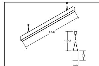
LED-Pendel-Profilleuchte direkt BIRO40. version: LED, Mounting method: Suspended, Place of installation: Ceiling-mounted, material: Aluminium / Acrylic, IP protection class: according to DIN EN 60529 IP20, Protection class: (EN 61140) I, voltage: 230V AC 50Hz, Power: 17,9W, Luminous flux: 1.430lm, Colour temperature: 3000K, Colour of light: white, Radiation angle: 80°, Adjustability: not adjustable, With operating gear, .
